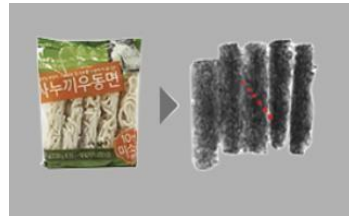
Detect foreign materials in packages with high-accuracy and non-destructive methods
