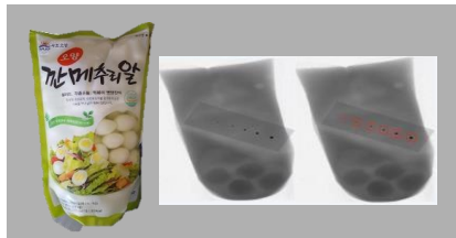
Detect foreign materials in packages with high-accuracy and non-destructive methods
